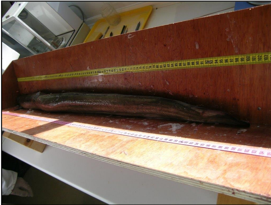
Figure 9.1. The ichthyometer used for the measurement of the total length of the eels.
